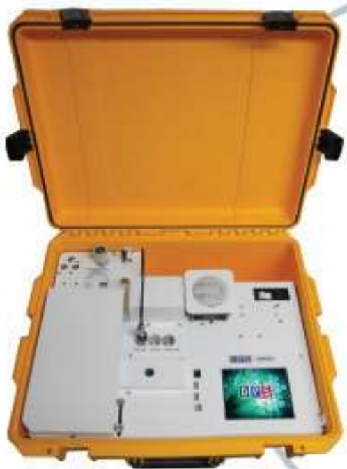
Companion 2 Portable GC With Dynamic Headspace Concentrator, (Vial Heater, "Cathedral" Trap, Sample Valve)
